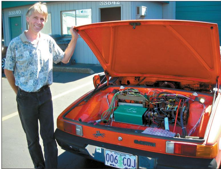
Otmar Ebenhoech shows off the Zilla converter in the trunk of his 1974 Porsche. Ebenhoech's Corvallis company, Electric Cafe, manufactures and repairs the converters that allow for high performance from batteries in electric cars. It can go from zero to 60 miles per hour in less than five seconds.
